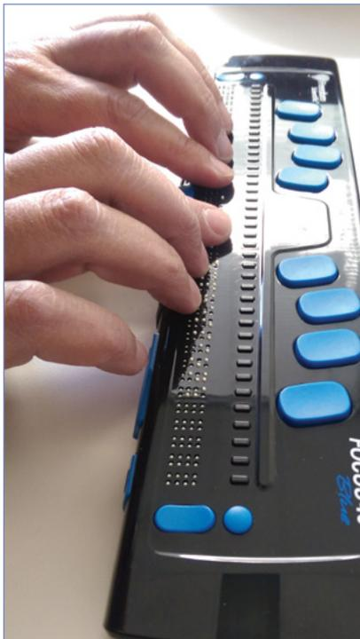
A refreshable braille display, upon which users can read using their fingertips. The braille text is displayed through a long matrix of pins that can be individually raised to form letters and words. Above the display pins on this photo are braille input keys. The braille display can be used in combination with a speech synthesizer, which converts text to speech.
